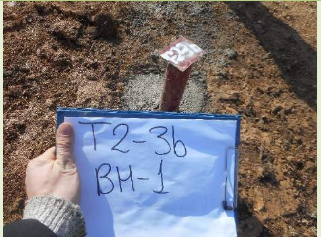
T2-3b BH-1, Piezometer
