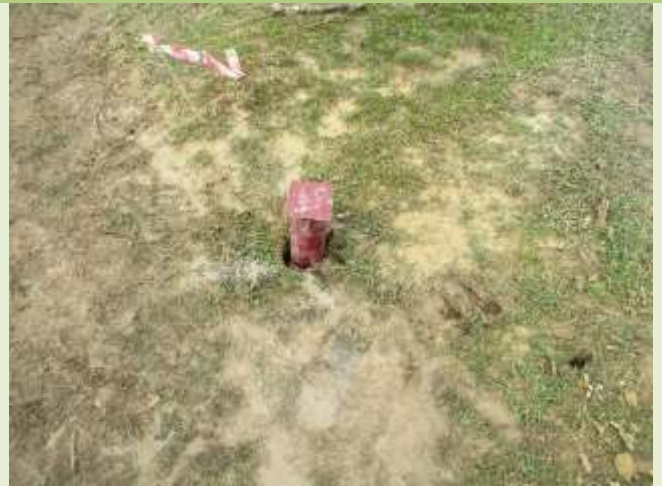
T1-3 BH-1, Piezometer
