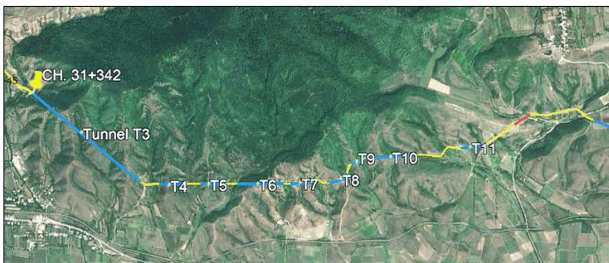
Figure 10. Tunnels and Channel Alignment 12
